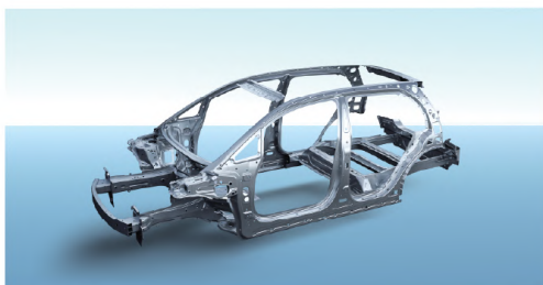
Safety body design High Strength steel comprising 71%
